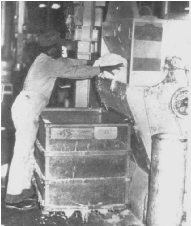
Figure 5 Worker loading chrysotile asbestos fiber by hand and without respiratory protection into the feed hopper of a carding machine at Marshville, NC, textile plant, prior to plant's acquisition and redesign by Raybestos Manhattan in 1969 (Lewinsohn et al. 1979)
